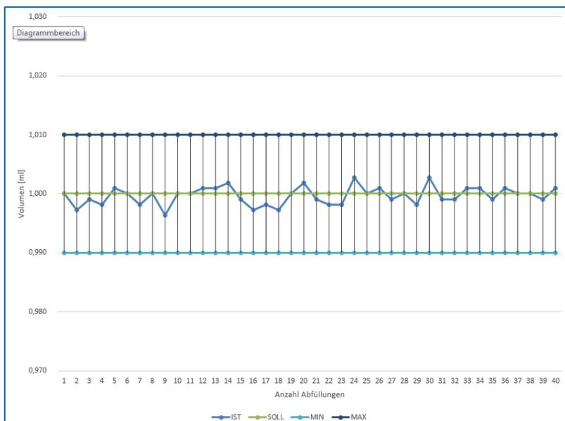
Illustration: Repeat accuracy for 40 fillings,  $x + 3\sigma = 1 \text{ ml} + 3 \times 0,0015$
