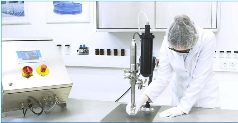
*Illustration: Semi-automatic filling using the Pharma Dispenser*
