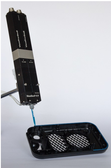
Picture 1: The special dosing geometry of the dispensers guarantees the pulsation free flow that is essential for precise control of mixing ratios.
