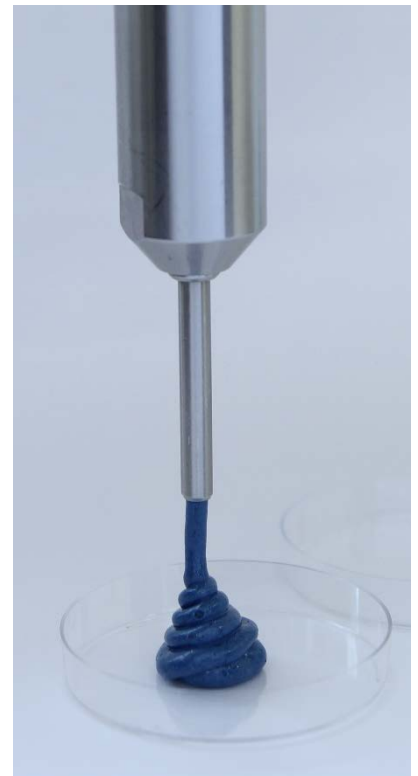
Figure 3: Dosing irrespective of viscosity using the Pharma Dispenser from ViscoTec
