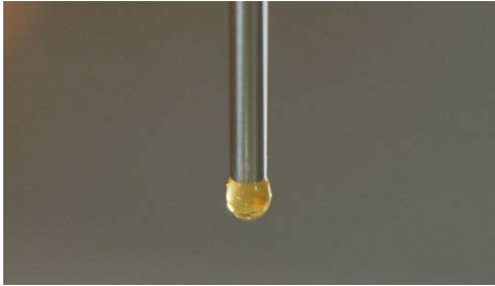
With the help of an adjustable suck-back option, dripping could be avoided after dosing.
